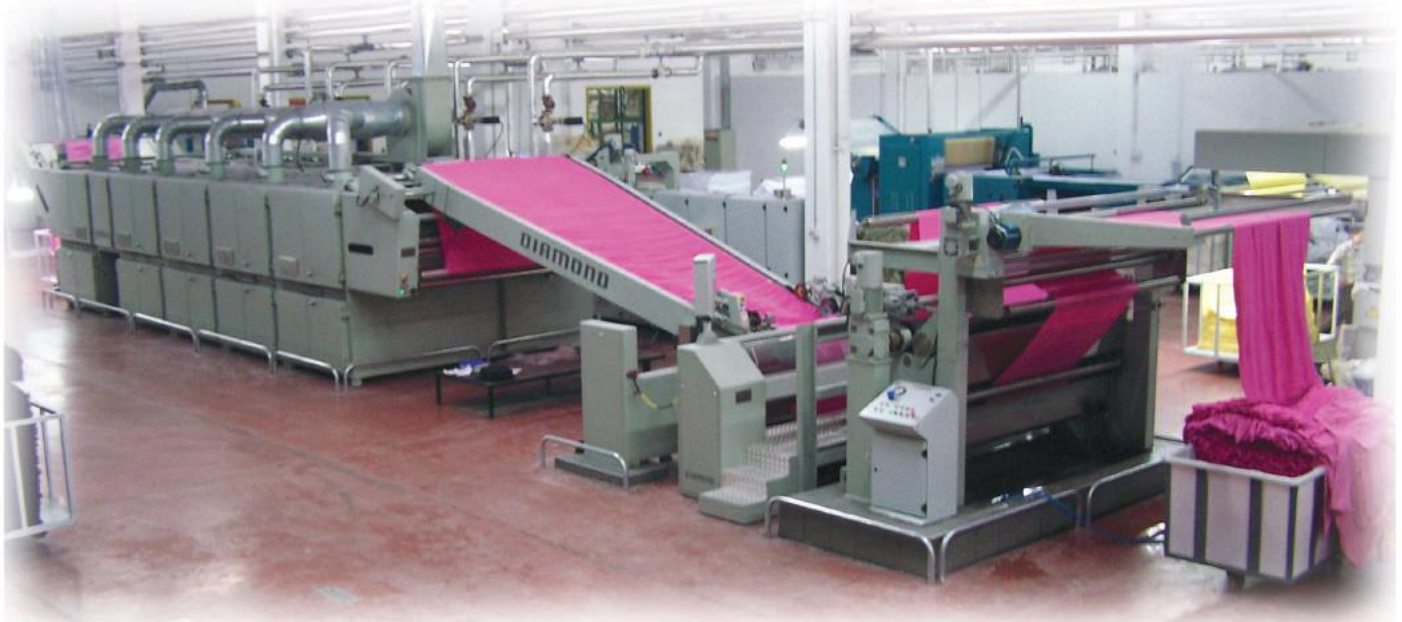
DRYMAX 5 KABİN TEK GEÇİŞ EGALİZE KURUTMA DRYMAX 5 CHAMBERS SINGLE PASS EQUALIZING ( pin-chain) DRYER
